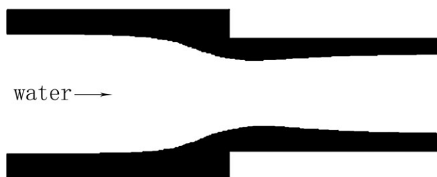
Figure 8. Residual wall thickness at upstream contraction transitions.
