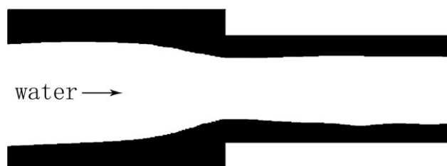
Figure 9. Residual wall thickness at downstream contraction transitions.
